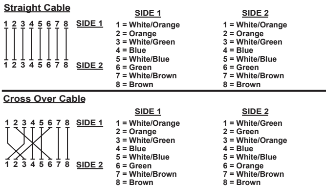
Figure A-1: Straight-through and Crossover Cable
