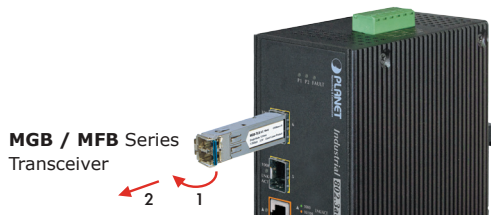
Figure 2-4: Pulling out from the transceiver
