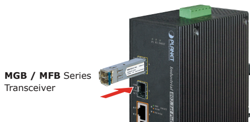
Figure 2-3: Plug-in the SFP transceiver
