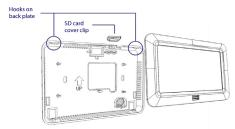
4. Make sure to connect the unit's 5-pin connector. Secure the front housing to the backplate by snapping it into place.
