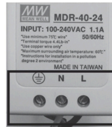
Figure 1. Connecting the 3 wires to the corresponding location.
